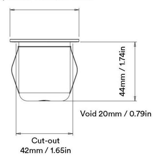
This product must be wired in Series, These products require an LED driver - DO NOT CONNECT DIRECTLY TO MAINS POWER! Connecting or disconnecting these luminaires while powered will damage the LED.
