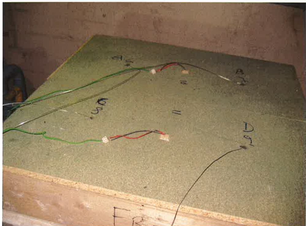
The unexposed surface of the ceiling directly after testing
