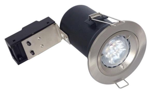
Fixed 90 min fire rated recessed downlight, integrated intumescent material completely seals the downlight and cut out in the event of a fire.
