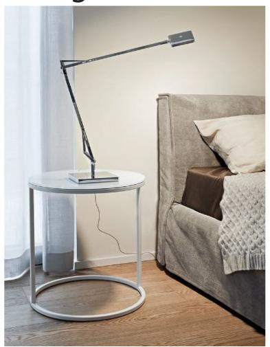
Adjustable Flos table lamp providing direct light. Aluminium painted or chromed body, with die cast head, joints and forks, and extruded arms. Diffuser in photoengraved polycarbonate and aluminate on the perimeter. Edge Lighting technology light source. Optical switch sensor placed on the head that provide 3-step dimming function and color temperature adjustment at 2700K or 3200K. Power cord length 150 cm. Plug-in power supply with interchangeable plugs.
